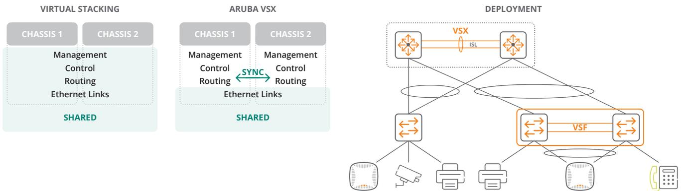
Figure 3: Comparison of Virtual Stacking and VSX
